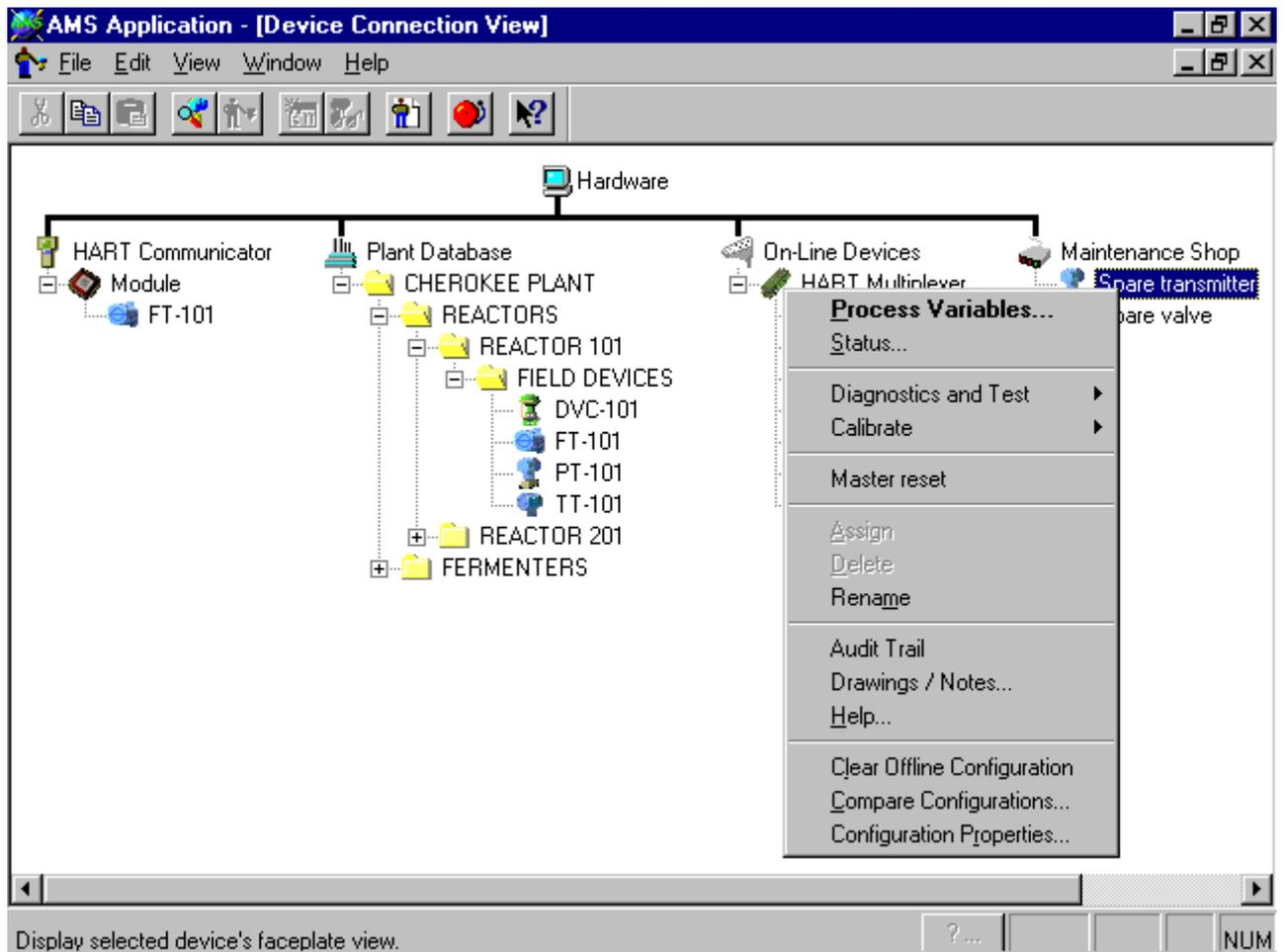
Figure 1. AMS gives users the ability to communicate with live instruments in the field, and to access all instruments' historical records. By simply clicking on an instrument icon all information, including device status, is instantly available.
